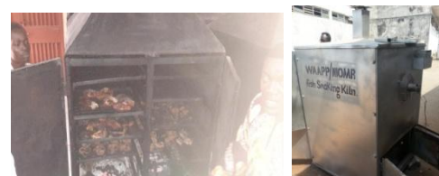
Fish smoking kilns developed by NIOMR and NSPRI
