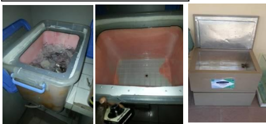
Cold boxes developed at NSPRI and NIFFR for keeping fresh fish for up to 14 days
